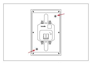
STEP 1: Remove the plastic screw(s) with a manual screwdriver. Do not use any electrical tools to avoid damaging the screw(s).
